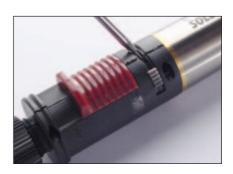
**9.** Reassemble your gas iron. Adjust the gas flow clutch (located under the gas flow slider) so that there is enough gas flow at lowest setting to light a small flame.
