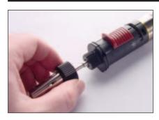
1. Start by taking off the tip assembly. This is done by unscrewing the metal barrel and plastic nut above the ignition switch.
