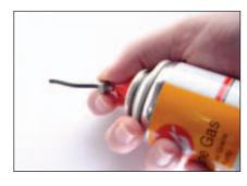
8. Using your butane gas refill can, insert at the hexagonal nut side and push repeatedly blowing out built up wax.
