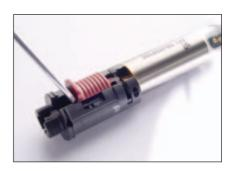
**6.** Wedge open one side of the plastic body (the opposite side to the screw holes.) Be careful not to break any parts off.
