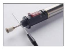
2. Un-screw the nozzle assembly by using the oxygen hole and a small screwdriver as a "T" bar.
