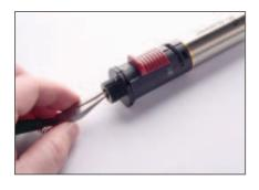
4. Carefully pull out the brass gas filter using long nose pliers.
