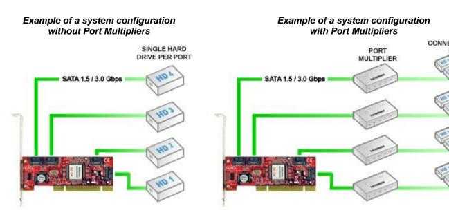
3. Port Multipliers reduce the amount of cabling required to connect an array of SATA devices.
