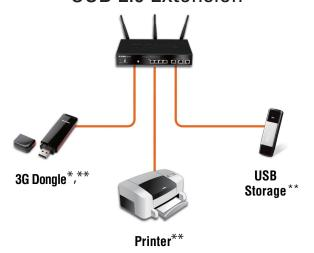
D-Link Unified Services Routers support USB 2.0 to extend functionality via Plug and Play.
