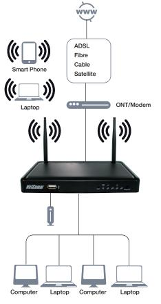
THE NETCOMM NP805N IS A FUTURE READY WIRELESS ROUTER THAT CONNECTS THE HOME OR OFFICE TO SUPER-FAST BROADBAND USING YOUR CHOICE OF AN ADSI. OR FUTURE FIBRE NETWORK CONNECTIONS.
