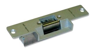
Ideal for use with the DIY Doorbell Video Intercom, the Swann Electric Door Strike allows you to open the door or gate with the touch of a button. The Swann Electric Door Strike is 12V operated and is fail secure so that it stays locked without power. Featuring a stainless steel faceplate and heavy-duty latch, the Swann Electric Door Strike will mount in most wood or aluminium frames.
