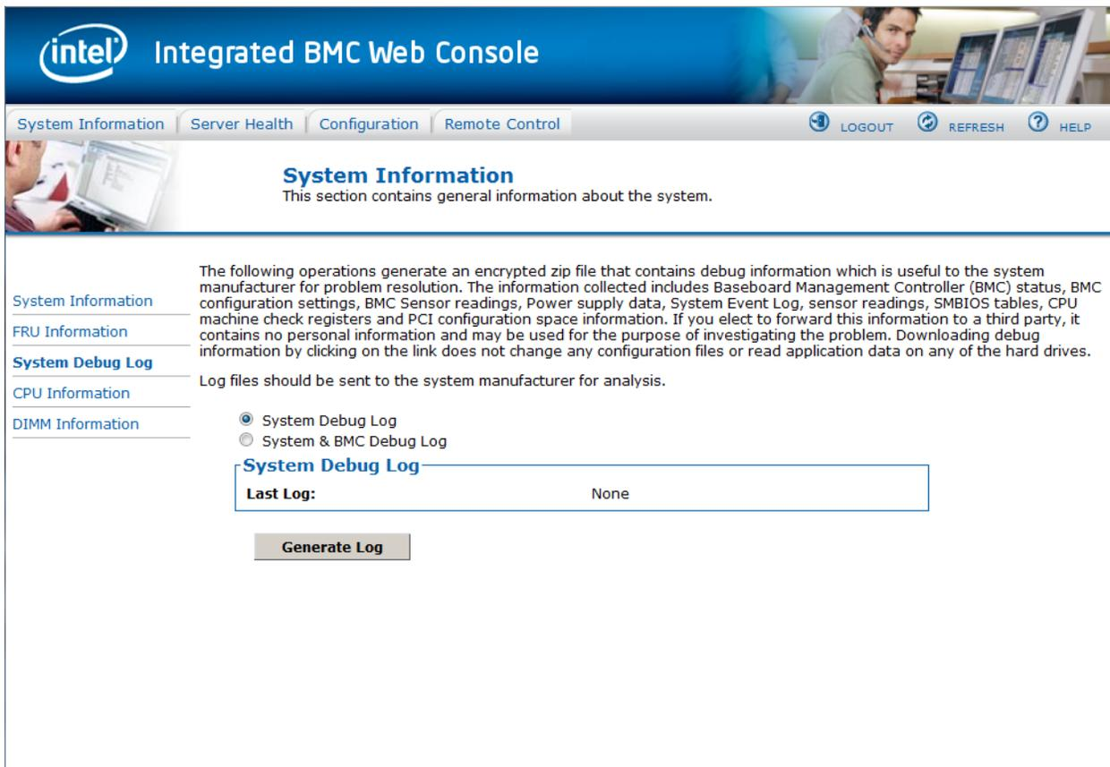
**Figure 51: System Debug Log Page on EPSP Platforms Based on Intel® Xeon® Processor E5-4600/2600/2400/1600/1400 Product Families**
